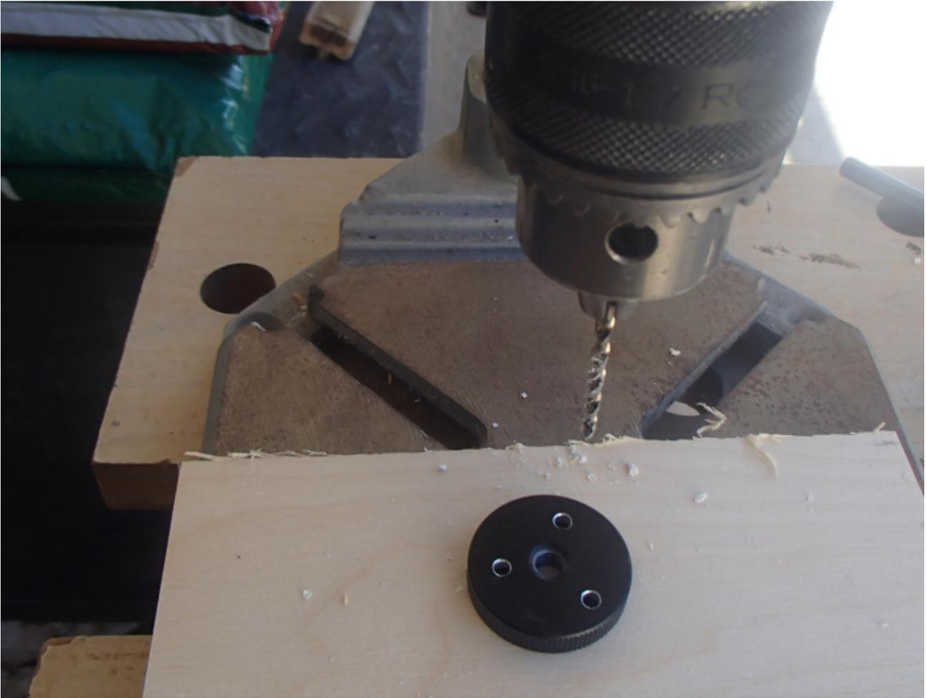
Chamfer them at 45° for the 3 mm countersunk wood screws. (I used this red tool and get a painful tendinitis – Rather use a chamfering drill)
